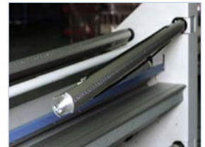
Cantilevered Supply Shaft*
